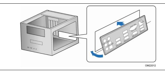
Figure 4. Installing the I/O Shield
